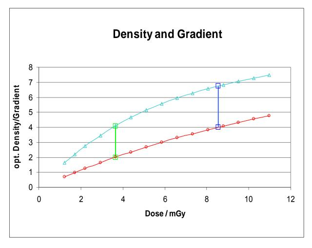
**Figure 1:** Mean opt. density  $\langle D-D_0 \rangle$  (red curve) and mean gradient  $\langle G \rangle$  (blue curve) of eight films as function of exposure dose K.
